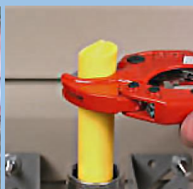
4. The pipe end should be cut squarely.
